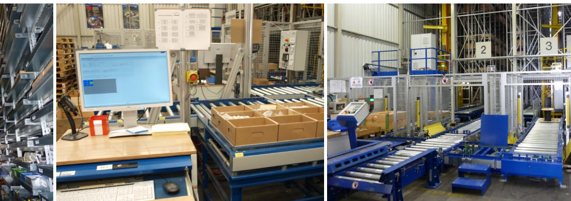
Kommissionierplatz Tablarlager. Picking workstation at the tray warehouse.
